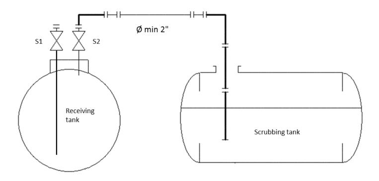
S1 is a liquid phase valve and S2 a gas phase valve.
